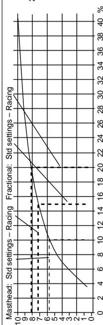
Note: For 2 mm wire, use 2,5-slot and read SureCheck scale + 3. 100% = 310 Kg/680 lb.
